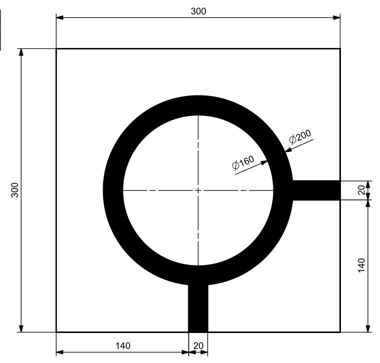
300 Tile: Pacman Roundabout Tile number: 50 All dimensions in mm Ø200 300 140 140
