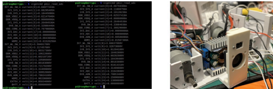
Figure 5: Voltages before and after step-down adjustments | Active cooling for 12 A step-down converter
